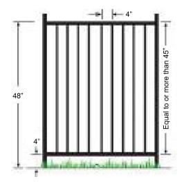
•Where the barrier is composed of horizontal and vertical members and the distance between the tops of the horizontal members is less than 45", the horizontal members shall be located on the swimming pool side of the fence.
