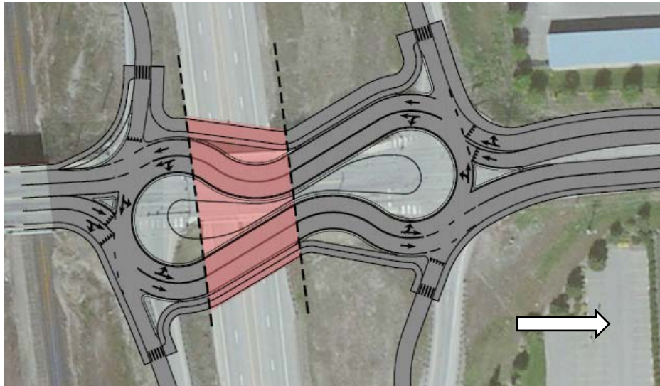
Figure 3-8: Dog Bone Roundabout Option 2
