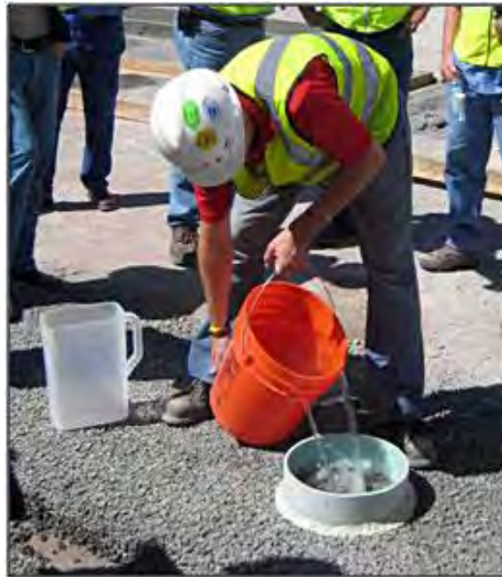
Figure 5: Application of water in a single ring infiltrometer test (NRMCA 2015)
