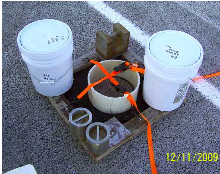
Figure 6: Use of neoprene gasket and a weighted cylinder to provide for a tight seal (Brown and Borst 2014).
