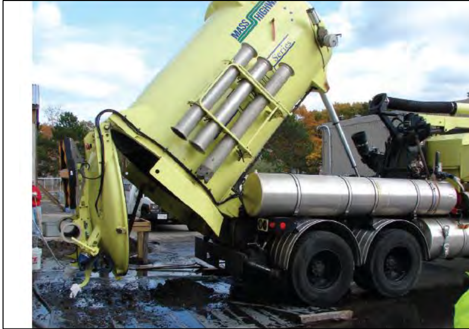
Figure 7.3 Example of vacuum truck emptying the catch basin contents onto a tarp prior to processing the material
