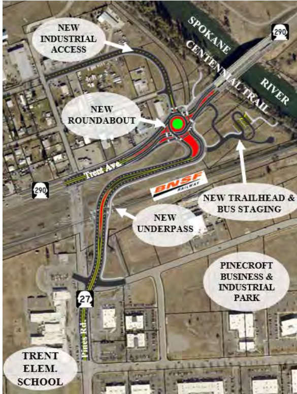
Figure 1: Pines Road/BNSF Grade Separation Project
